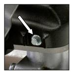
Fit the saw on the spindle by reversing the sequence. Make sure that the holes in the saw blade point upwards! To make it easier to change the blade, use the spindle lock to clamp it.
